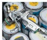
Jason Wilkins keeps his SATA spray gun in a locked strongbox, in a locked paint room, in a locked workshop building. That and its as-new condition (it's eight years old) should tell you how much he cares for it. 'DeVilbiss make very good guns, but only SATA actually grind in the needle to the fluid tip and test each gun. The fan they produce is totally consistent. You can buy the whole gun for £400-£500 or new air caps, or tips and needles for about £130. Bargain.'
